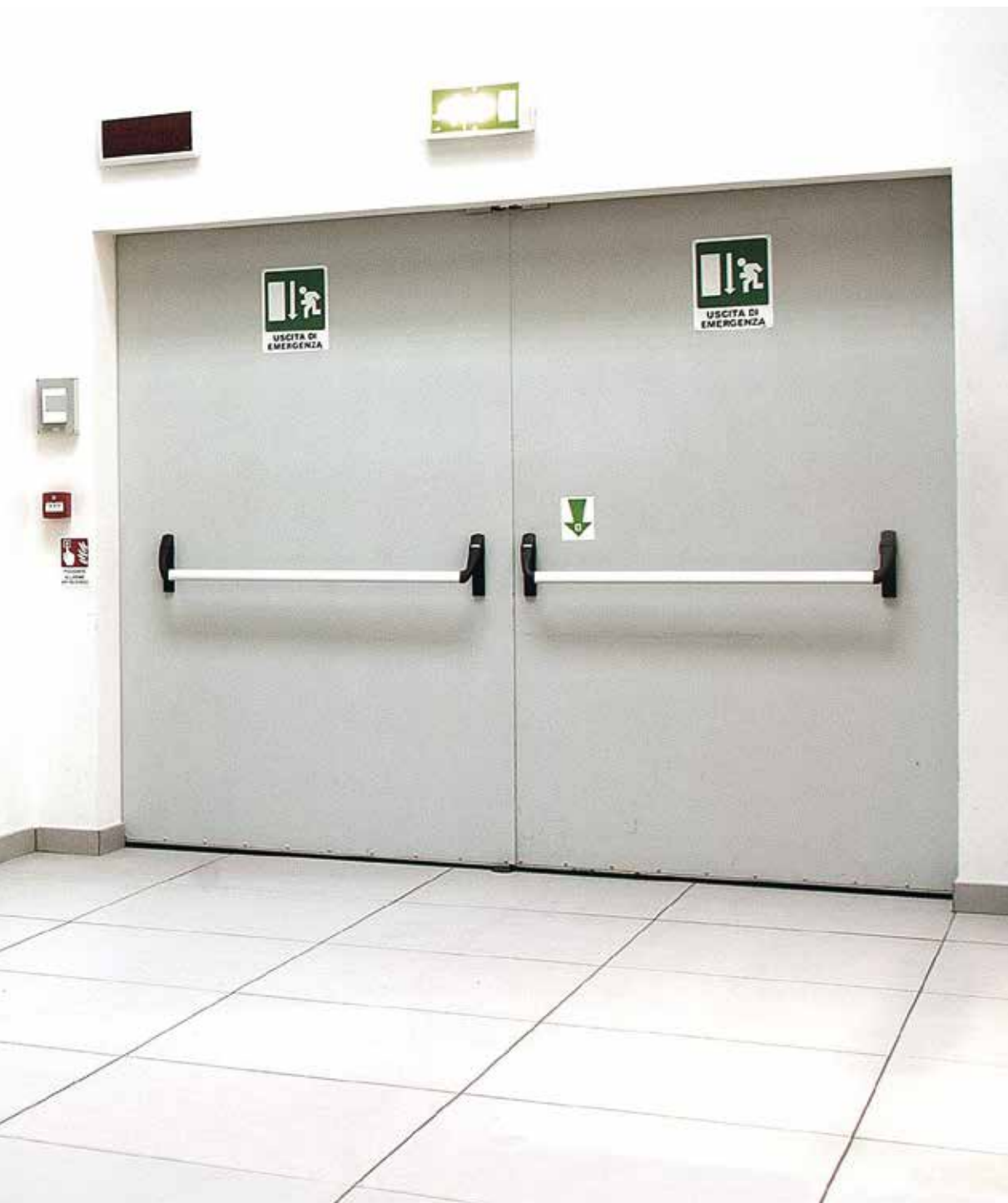
metal collection Art. 11M EI 60 porta a battente 2 ante simmetriche double symmetric fireproof door pannello in metallo preverniciato in colori RAL metal door panel prepainted in RAL colours SP. TH. 8/10 maniglione antipanico a leva panic bar exit device chiudiporta a slitta sequenziale sequential doorcloser cassa in metallo - metal doorframe SP./TH. 15/10 verniciata a polveri RAL - powder coating RAL Mod. PM1TB
